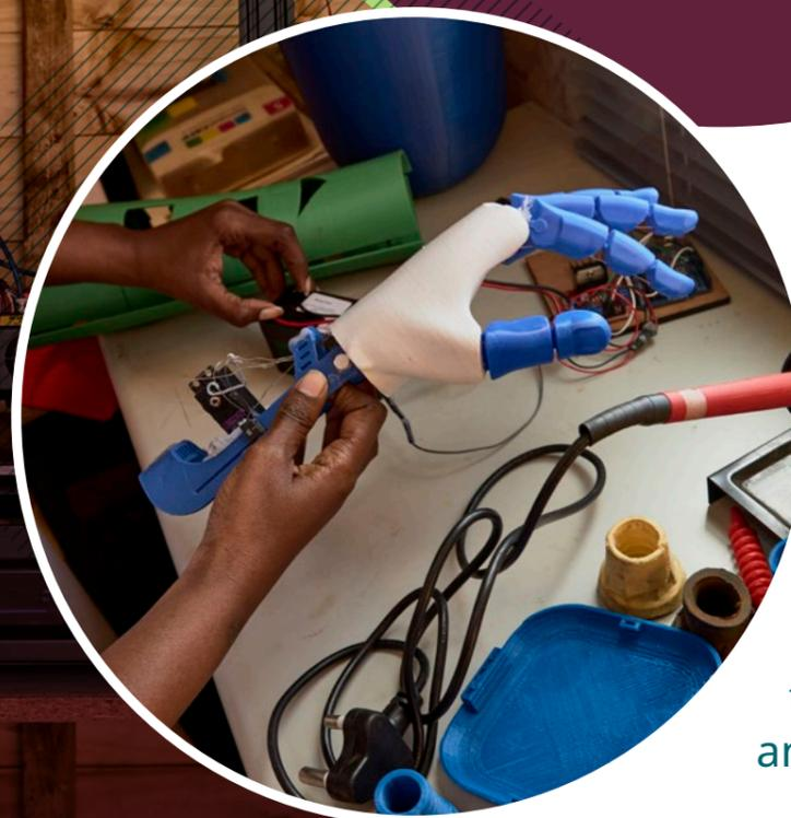
Using 3D printing technology and plastics that are recycled and collected locally, Uku'Hamba Prosthetics and Orthotics create unique, lightweight prosthetics in bold styles, giving users access to empowering prosthetics that delight, at a fraction of the cost to both users and the environment.
